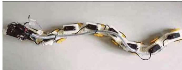
A prototype of the snake robot created by International Islamic University Malaysia lecturers. The snakebot can be used in impenetrable spaces, like a collapsed tunnel or to slither over earthquake rubble. Bername PIC
